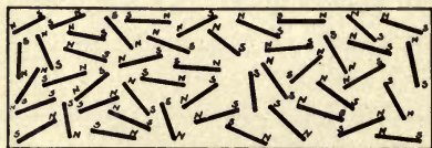
FIGURE 132.—ARRANGEMENT OF MOLECULES IN A PIECE OF IRON NOT MAGNETIZED.
